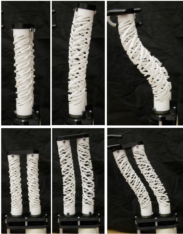
Fig. 3. Demonstration of a linear actuator created by a pair of handed shearing auxetic cylinders (HSA). Linear extension and compression is achieved just by the use of a single servo. Compliance is created due to the flexible nature of the PTFE tube that the HSA is patterned into.
